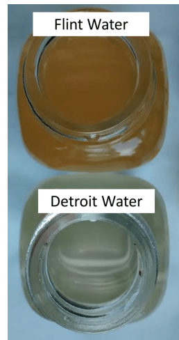
Figure 3: Higher release of iron is evident in the Flint water glass reactor containing iron than that with Detroit water
